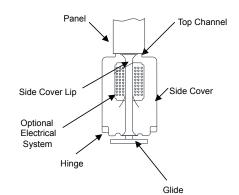
FIGURE 1 Cable Management Channel
