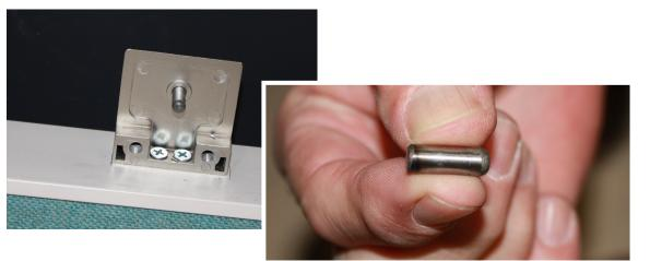
6. Establish your hole location. Mount the block using 2 1" Phillips screws.
