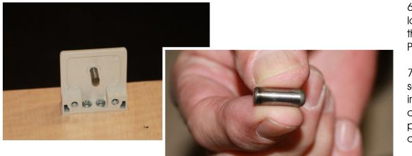
6. Establish your hole location. Mount the block using 2 1" Phillips screws.
